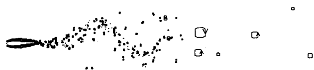
Fig. 9 Distribution of vortices at time t = 15 ; K = 1.0 , \sigma = 0 , h = 0.05 , \zeta = 0 deg, \alpha = 0 deg (the size of the vortex represents its strength; for larger vortices, the direction of rotation is shown by the arrows).
